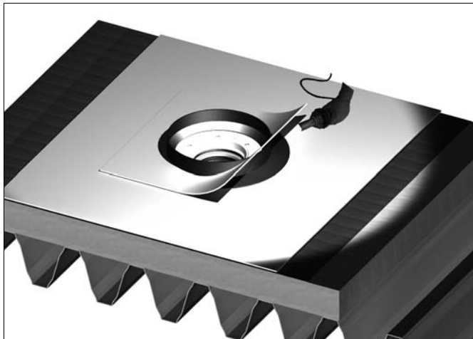
Illustration 10.58 Installing the PVC patch
